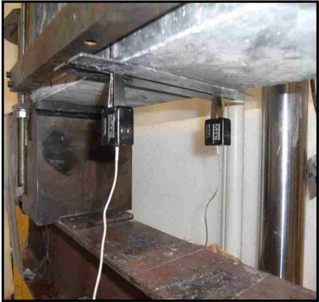
Figure 3.22: Attachment of clip gages to the knives
