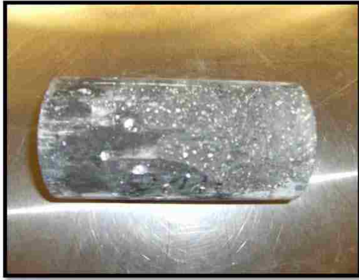
Figure 3.4: The UHPC specimen after the compression test
