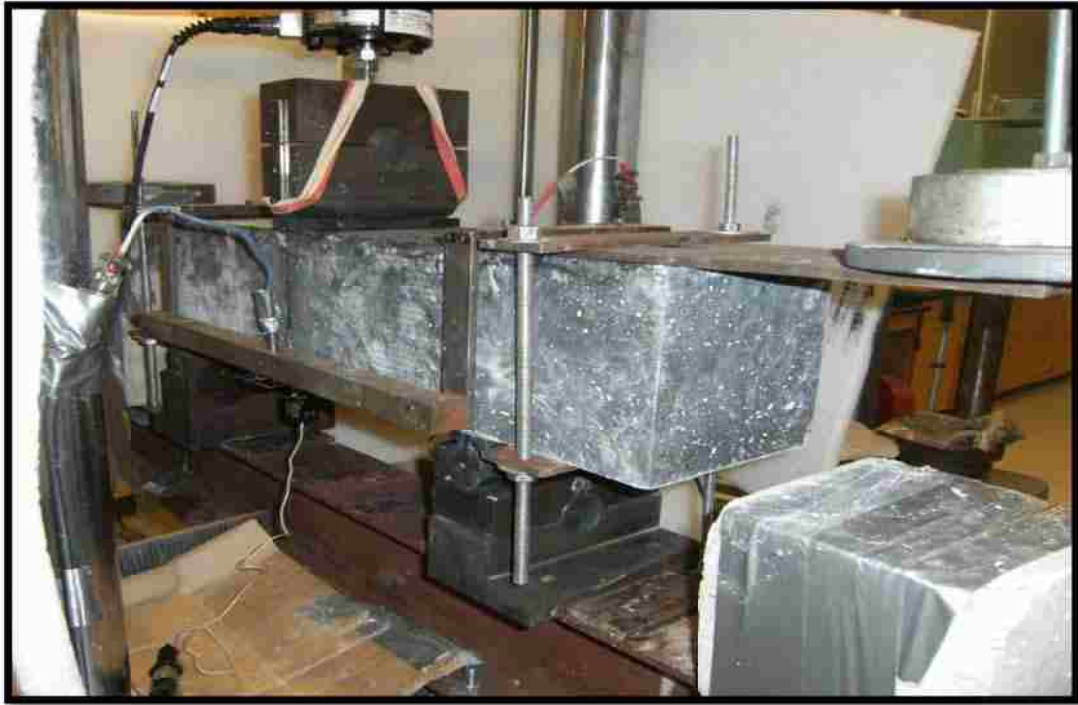
Figure 3.24: The final beam setup for starting the test
