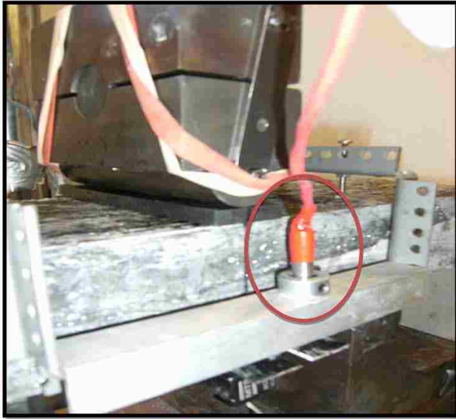
Figure 3.23: Placement of LVDTs in the frame
