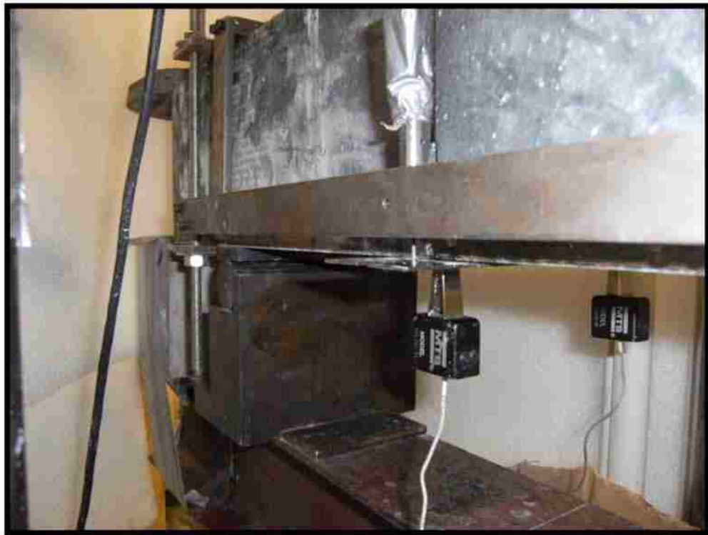
Figure 3.20: View of the specimen, with the CMOD gage in the center, and the mounting plates with wings to provide support for the mobile tips of the displacement transducers
